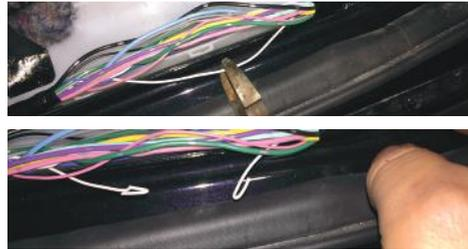
9. Locate the single white wire in the vehicle loom. Test that it signals +12V when the brake pedal is depressed.
