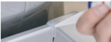
6. Apply silicone sealant to the bed's front corners to protect against water ingress. Use clear or black depending on vehicle shade.
