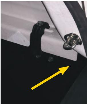
4. Pass the wires for the brake light (located at the rear driver's side of the canopy) through the gap under the vehicle's side rail.
