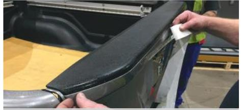
4. Carefully apply the tape, where the door seal touches, removing any bubbles as you go. Use a squeegee if possible.
