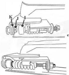
tighten the nut (E) till bush (I) completely cover the bolt head (J) and touch the flat washer (K)
