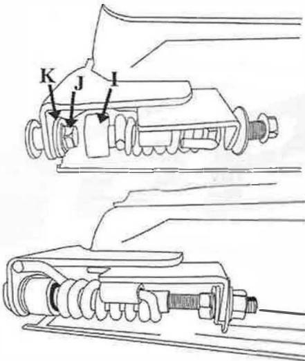
tighten the nut (E) till bush (I) completely cover the bolt head (J) and touch the flat washer (K)
