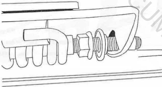
4.3 tighten nut (E) while holding the rod of the spring set with #6 wrench (F)
