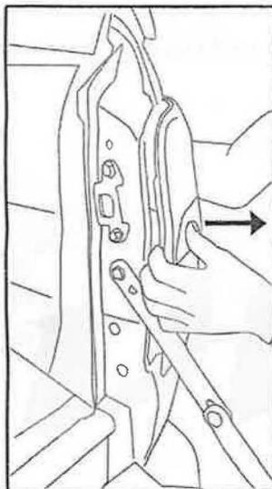
8. Attache damper to the truck using original bolt (R) (S)
