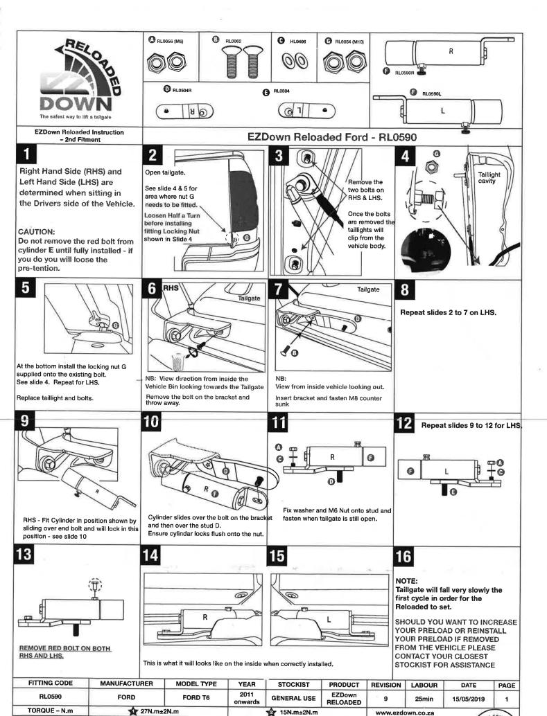
NB: After installation please close tailgate gently to ensure that there is no interference with any hardware.
