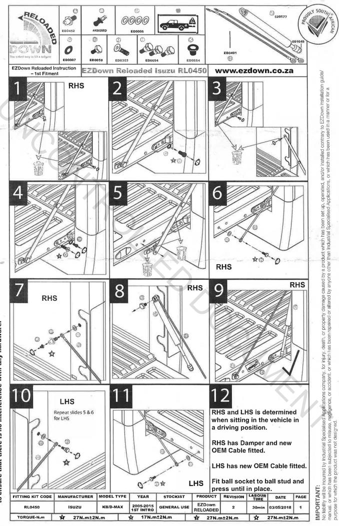
NB: After installation please close tailgate gently to ensure that there is no interference with any hardware.
