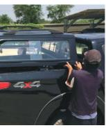
14. NOTE: The canopy may sit a little 'high' until the clamps have been applied. Set the position as shown below, adjustment may be required later.
