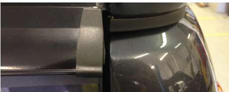
17. Centralise the bottom of the rear door to the tailgate.
