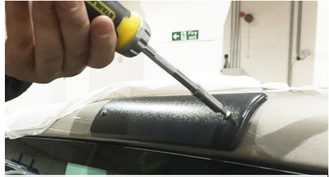
10. Fit the blanking plate supplied.
