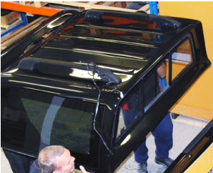
14. Lift the canopy on to the bed of the vehicle.
