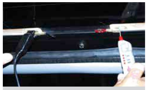
2. Switch on the vehicle's heated rear screen and check there is +12v across the element on the hardtop door.
