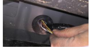
13. Underneath. make a small hole in the grommet and pass the section of harness containing the grey and yellow wire through into the passenger compartment.
