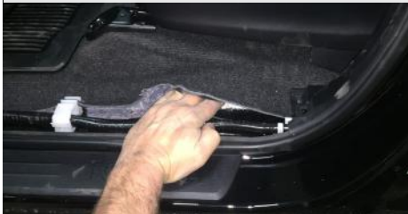
14. Reach under the carpet and lining to locate the wires.
