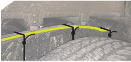
9. Take the other end of the harness forward, along the top of the N/S chassis rail.
