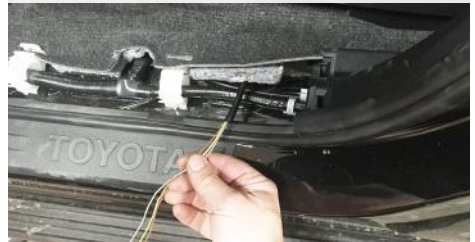
15. Draw the wires through and take them forward through the white clips.
