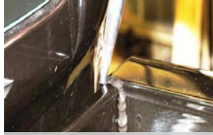
12. Fill the joint between the front and side rails with silicone.
