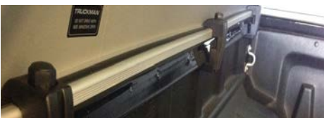
17. Centralise the bottom of the rear door to the tailgate.
