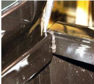
14. Fill the joint between the front and side rails with silicone.
