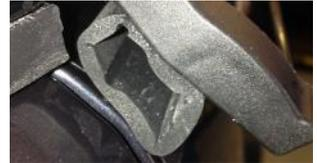
23. Ensure the rear door fully latches when closed firmly (the seal under the door should now be half compressed).
