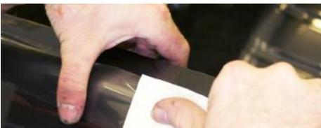
29. Carefully apply the tape, where the door seal touches, removing any bubbles as you go. Use a squeegee if available.
