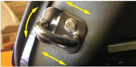
24. Small adjustments can be made, if required, by re-positioning the striker plates.
