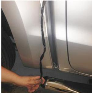
35. Pass the canopy wiring harness down between the cab and the load bed.
