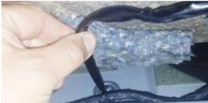
40. Draw it through under the drivers seat and under the carpet to the driver's sill.
