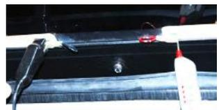
47. Switch on the heated rear screen and test for 12v across the element.
