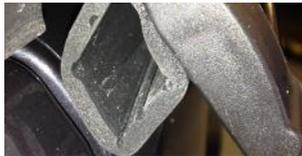
17. Carefully adjust the position of the canopy so that the seal under the rear door is just in contact with the tailgate.
