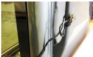
7. Temporarily tape the canopy wiring harness to the roof bar.
