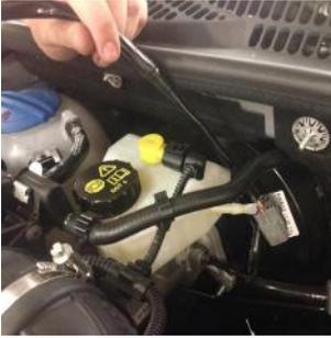
31. Locate the wiring harness from the fitting kit then, in the engine bay, pass the grey plug down to the chassis in the position indicated by the white arrow.
