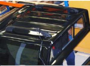
16. With the tailgate closed, lift the canopy on to the bed of the vehicle.
