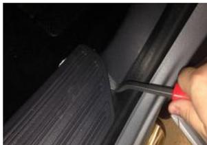
38. Carefully unclip the sill trim from the driver's door.
