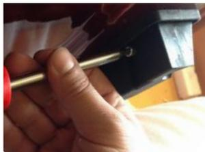
5. Remove the roof bar retaining screws.
