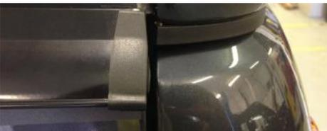
19. Centralise the bottom of the rear door to the tailgate.
