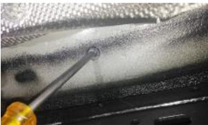
37. Make a hole in this grommet located below the driver's seat.
