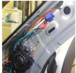
44. Bring the wires for the brake light and heated screen up to the 'A' post and make the connections as shown in the guide above.
