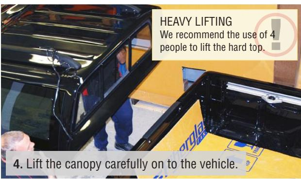
4. Lift the canopy carefully on to the vehicle.
