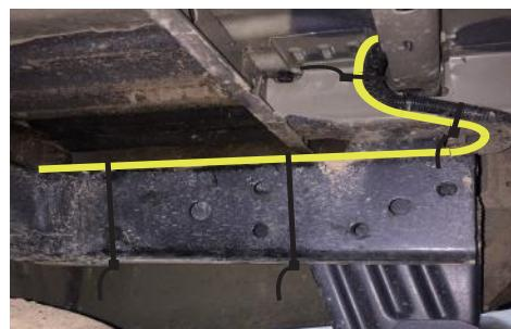
7. Feed the harness down to the chassis following the vehicle's wiring loom.
