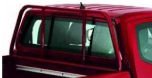
5. If a guard frame is fitted behind the cab, extract the screws and remove it. REPLACE THE FIXINGS
