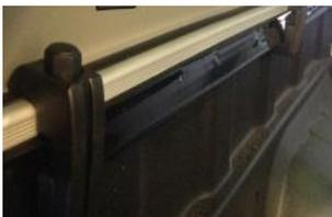
4. Assemble the clamps loosely in position on the side rails. There are gaps in the rubber trim in each position.
