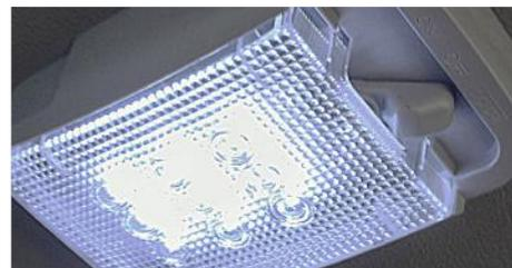
4. Switch the interior light to 'Door'. Check it goes out when the rear door is shut.
