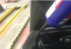
1. Just before fitting the canopy, fill any gaps between the front and side rails with sealant.
