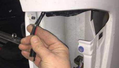
6. Draw the harness through into the light recess leaving approx 100mm of cable inside the load bed.
