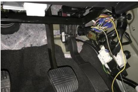
Connections to the vehicle are in the driver's sill as for the double cab except for the Yellow and Grey wires which are connected in the drivers side kick panel (adjacent to the accelerator pedal). Refer to the table above for expected wire colours. Test wire function before connection.
