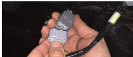
1. Connect the two parts of the loom together ensuring the cable and plug are secured tidily (cable tie to the rear clamp). Re-connect the vehicle's battery.
