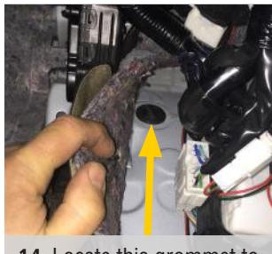
**14.** Locate this grommet to the right of the accelerator pedal.
