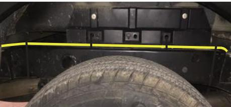
9. Cable tie the harness to the top of the chassis rail up to the front of the rear wheel arch
