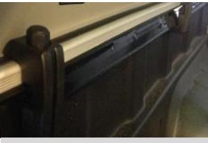
4. Assemble the clamps loosely in position on the side rails. There are gaps in the rubber trim in each position.
