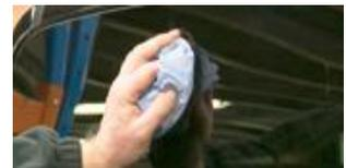
6. Thoroughly clean the vehicle's rear window and the top surface of the bed rails
