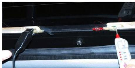
2. Switch on the vehicle's heated rear screen and check there is +12v across the element on the hardtop door.
