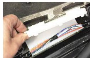
**20.** In the driver's sill open the cover of the white plastic box exposing the wires inside.
