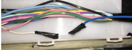
25. Insulate both sections of wire and secure before closing the box.
