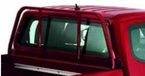
5. If a guard frame is fitted behind the cab, extract the screws and remove it.
