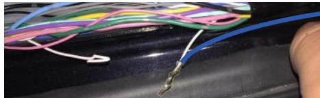
24. Solder the blue wire to the section of white wire which leads forward.
