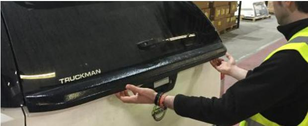
2. The rubber seal on the bottom of the door should just be in contact with the tailgate spoiler.
