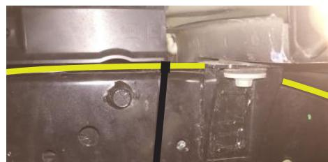
9. Cable tie the harness to the top of the chassis rail up to the front of the rear wheel arch
