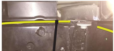
10. After which it is fastened to the vehicles wiring loom on the side of the chassis rail.
