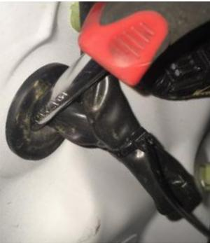
**18.** Locate the grommet pictured in step 14, make a small hole and pass the leg of the harness containing the green, yellow, grey, brown and blue wires through into the driver's foot well.
