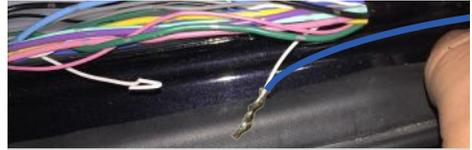
24. Solder the blue wire to the section of white wire which leads forward.
