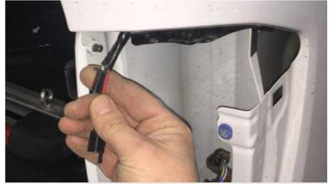
6. Draw the harness through into the light recess leaving approx 100mm of cable inside the load bed.
