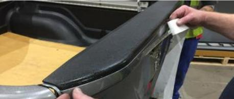
4. Carefully apply the tape, where the door seal touches, removing any bubbles as you go. Use a squeegee if possible.
