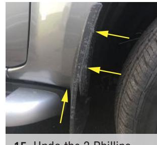
**15.** Undo the 3 Phillips retaining screws on the O/S/F mud flap.
