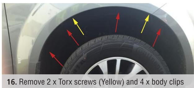
**16.** Remove 2 x Torx screws (Yellow) and 4 x body clips (Red) from the wheel arch liner.
