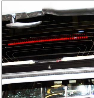
**11** Use a multimeter (if available) to confirm a current across the heated rear window when on.
