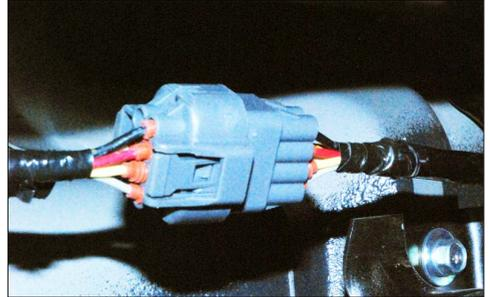
**8** Insert the fuse into the fuse holder and connect the wiring loom to the hardtop.
