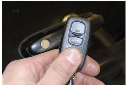
**12** Check that the hardtop locks and unlocks with the vehicle's remote.
