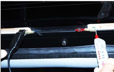
**9** Open the hardtop door. Ensure the light is set to "Door" and that the interior light is on. Close the door and check it switches off.
