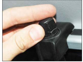
(Just more than hand tight / 8Nm Torque)
