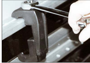
(Just more than hand tight / 8Nm Torque)
