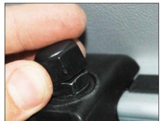
(Just more than hand tight / 10Nm Torque)
