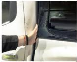
**5.** Line up the front of the canopy with the front of the vehicle's bed rail.
