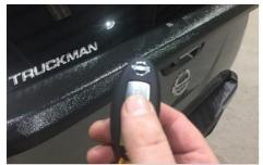
5. Close all of the doors and check that the canopy locks and unlocks with the vehicle's remote.
