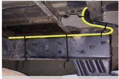
**8.** Run the harness forward, along the O/S chassis rail using the large cable ties.
