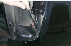
**7.** Feed the harness down to the chassis following the vehicle's wiring loom.
