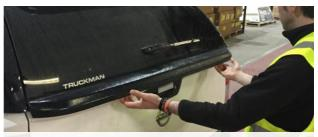
2. The rubber seal on the bottom of the door should just be in contact with the tailgate spoiler.
