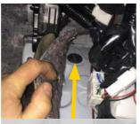
**14.** Locate this grommet to the right of the accelerator pedal.
