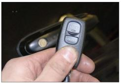
Check that the hardtop locks an unlocks with 12 the vehicle's remote.
