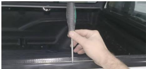
17. Insert the frame in the canopy then secure it with the centre screw.
