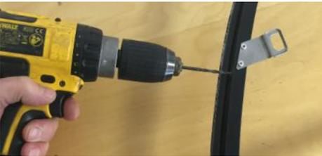
14. Open the holes in the frame to 3.5mm to prevent the screws from binding.
