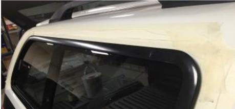
1. Apply masking tape around the frame to protect the paintwork.
