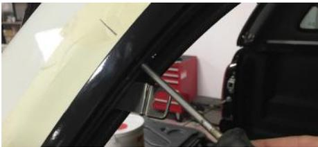
5. Carefully remove the screws taking care not to damage the heads.
