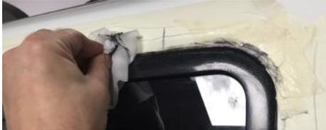
20. Check the windows slide and lock correctly then wipe off the excess sealant-
