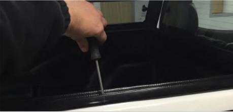
9. Locate, mark and remove the final centre screw.
