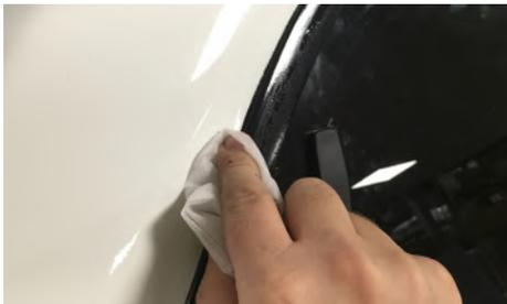
22. Use silicone or multi-purpose wipes for the final finish. Check there is a continuous fillet of sealant along the top and sides of the window. If necessary, apply a little more sealant then clean-up using the wipes as before.
