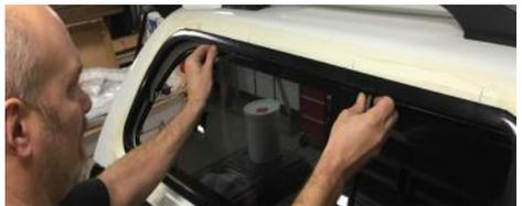
8. Ease the top of the frame out of it's recess then, stretching the frame slightly, remove both pieces of glass.
