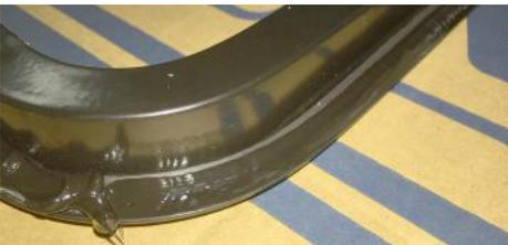
16. Apply a generous bead of sealant around the top and sides of the frame.
