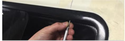
19. Insert the remainder of the screws making sure the heads will not foul the glass. (use fresh ones if the heads of the old ones are damaged)
