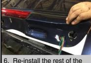
6. Re-install the rest of the cables into the spoiler.
