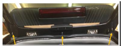
1. Unscrew the 10mm hex screws indicated in the picture above. Release the spoiler and place upside down on the roof of the hardtop.
