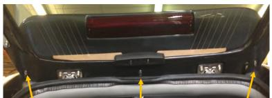
1. Unscrew the 10mm hex screws indicated in the picture above. Release the spoiler and place upside down on the roof of the hardtop.
