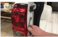
3. Locate and remove the rear light cluster retaining screws
