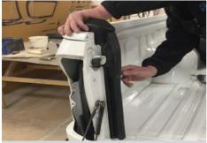
5. With liner removed, offer up the units to the vehicle as shown
