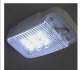
46. Replace the fuse then open the rear door. Ensure the switch is set to "Door" and that the interior light is on. Close the door and check it switches off.
