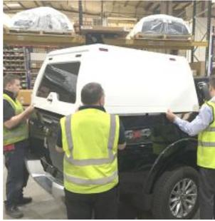
**12.** Line up the front edge of the canopy with the front edge of the vehicle's bed.
