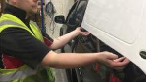
**14.** Close the rear door and check the lower seal is touching the tailgate.
