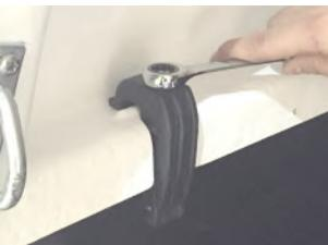
**17.** Re-check the position of the canopy and door. If necessary, slacken off the clamps, adjust the position and re-tighten them.
