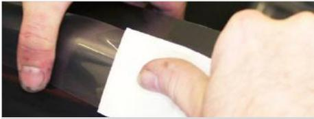
21. Carefully apply the tape, where the door seal touches, removing any bubbles as you go. Use a squeegee if available.
