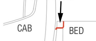
**7.** Seal the vertical joint between the moulding and the vehicle body. Continue the sealant down to fill the small gap in the vehicle bodywork below the moulding.
