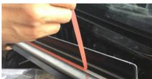
**5.** Locate the bulkhead moulding in the box base and remove the backing from the adhesive tape.
