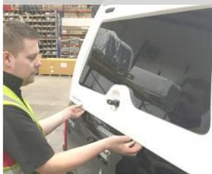
**15.** Assemble the clamps, as shown, in the recesses of the side rails.
