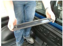
3. Screw the blanking plate to the back of the cab using the original screws. Place the light in the glove box for later use. Clean the cab window
