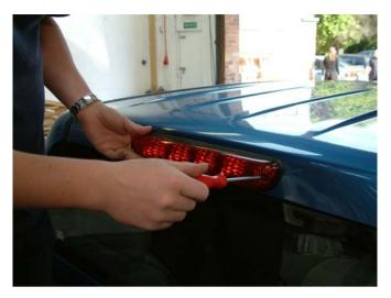
2. Peel the water seal from the back of the light and place it on the blanking plate as shown
