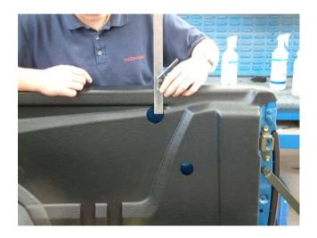
11 The front holes should be positioned 310mm from the front of the **loadliner**. The rear holes should be 290mm from the rear of the **loadliner** as shown below. The centre holes should be mid-way between the above two sets of holes
