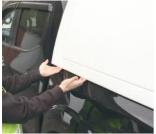
9. Adjust the position of the hardtop so that the overhang is equal on both sides.
