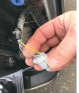
6. Solder the canopy's brake light wires to the vehicle's wireing using the colour guide below.
