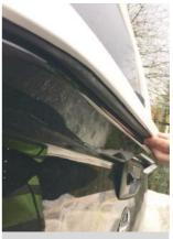
8. Align the top centrally and ensure that the seal under the hardtop door is just touching the tailgate.
