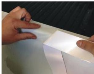
23. Carefully apply it to the tailgate where the door touches, rubbing outwards to remove any bubbles as you go.
