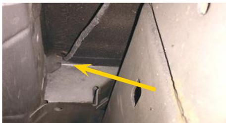
8. Drill a hole in the vehicle's floor in the location indicated above, treat with rust inhibitor and fit a grommet.
