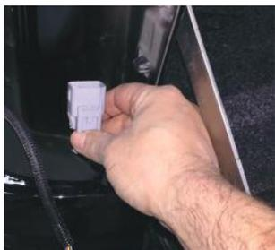
4. Draw the plug up through the light recess and through the gap under the vehicle's rail into the load bed.
