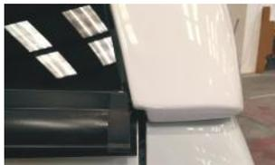
11. Finally, check that the seal under the rear door is just in contact with the tailgate.
