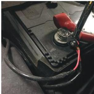
11. Take the section of harness containing the red and black wires forward along the chassis then up into the engine bay.
