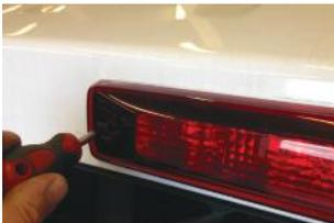
2. Unscrew the vehicle's third brake light and pull it away from the bodywork.
