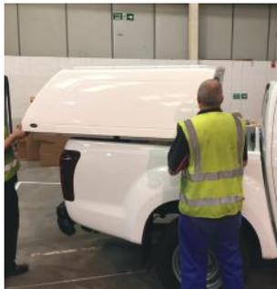
8. Begin positioning by lining up the front edge of the hardtop with the front edge of the load bed.
