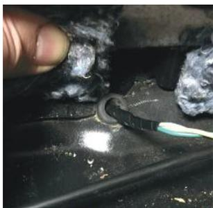
9. Pass the harness through the grommet, into the interior of the vehicle.
