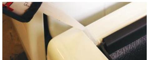
5. Fill the front corners of the bed with silicone sealant. (Where the side rails meet the front rail).
