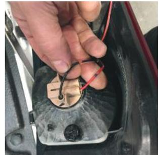
19. Test the brake light function before replacing the rear light cluster. Secure any loose wiring with cable ties. Finally, re-test the light and check the clamps.
