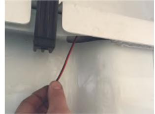
16. Locate the brake light wires and pass them through this aperture into the rear wing.
