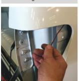
17. Draw the wires through into the rear light cluster recess.
