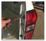
14. Remove the 2 retaining screws from the O/S rear light cluster.
