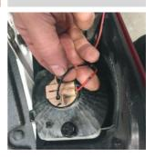
19. Test the brake light function before replacing the rear light cluster. Secure any loose wiring with cable ties. Finally, re-test the light and check the clamps.
