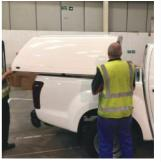
8. Begin positioning by lining up the front edge of the hardtop with the front edge of the load bed.
