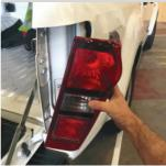
16. Locate the brake light wires and pass them through this aperture into the rear wing.
