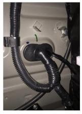
8. Locate the harness wires beneath the carpet under the seat and draw them to the sill area
