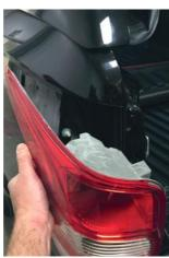
2. Locate the wiring harness in the fitting kit. From beneath the rear of the vehicle, pass the end up into the N/S/R light recess.
