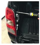
1. Remove the N/S/R light cluster fixings.
