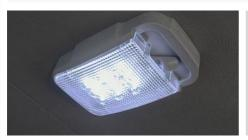
23. Switch the interior light to 'Door'. The unit will switch on and off automatically as the rear door is opened and closed.
