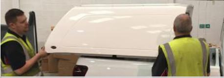
10. Lift the canopy on to the bed of the vehicle taking care that the front of the canopy is placed into the bulkhead moulding.
