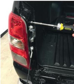
1. Remove the N/S/R light cluster fixings.
