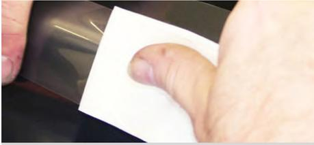
21. Carefully apply the tape, where the door seal touches, removing any bubbles as you go. Use a squeegee if available.
