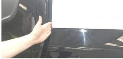
11. Line up the front edge of the canopy with the front edge of the vehicle's bed.
