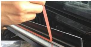
4. Locate the bulkhead moulding in the box base and remove the backing from the adhesive tape.
