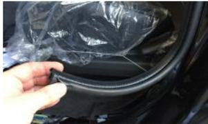
7. -and pull away the lower section of the B post rubber seal.
