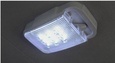
23. Switch the interior light to 'Door'. The unit will switch on and off automatically as the rear door is opened and closed.
