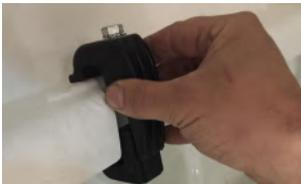
14. Assemble the clamps, as shown, in the recesses of the side rails.
