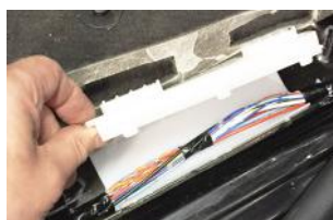
20. In the driver's sill open the cover of the white plastic box exposing the wires inside.
