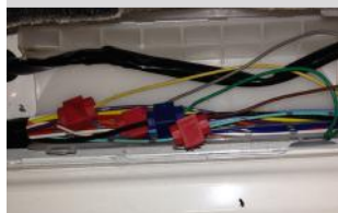
21. Either solder or use the connectors provided to attach the Yellow and Grey wires to the vehicles wiring loom (Refer to page 6).
