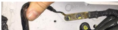
29. Attach the -Ve (Black) wire here. NOTE: Do not connect to the battery -Ve terminal.
