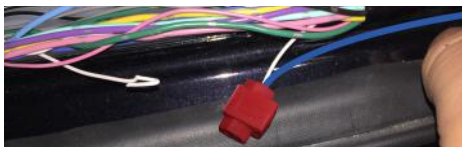
24. Use connector or solder the blue wire to the section of white wire which leads forward .
