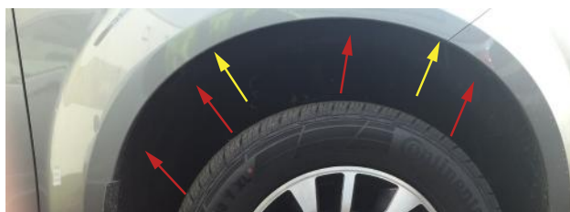
16. Remove 2 x Torx screws (Yellow) and 4 x body clips (Red) from the wheel arch liner.
