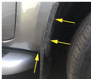
15. Undo the 3 Phillips retaining screws on the O/S/F mud flap.
