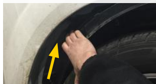
17. Run the wiring harness along the vehicle loom and up behind the wheel arch liner.
