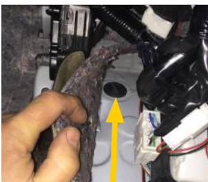
14. Locate this grommet to the right of the accelerator pedal.
