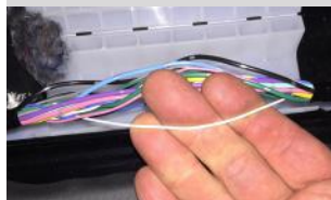
22. Locate the single white wire in the vehicle loom. Test that it signals +12V when the brake pedal is depressed.
