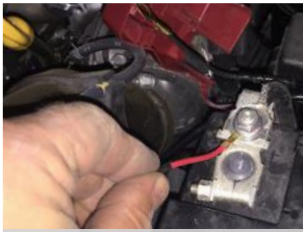
3. Battery +Ve connection.
