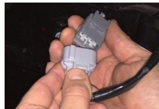
8. Connect the harness to the canopy plug.
