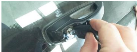
2. Push the small button on the left of the handle to open the key cover. Insert the key, ensure it is turned fully clockwise then remove it. This operation engages the keyless remote locking.
