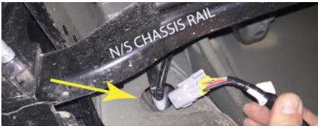
4. Take the wiring harness from the fitting kit then, from underneath the N/S rear of the vehicle, pass the grey plug up through this hole, into the light recess.
