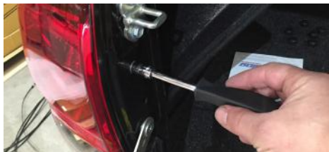
4. Replace the rear light and all of the interior trims. 5. This completes the installation of the optional electrical package.
