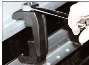
(Just more than hand tight / 8Nm Torque)
