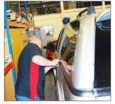
4 Align the top centrally on the bed. Ensure there is a gap between the hardtop and the cab, and that the lower door seal is hard up against the tailgate.
