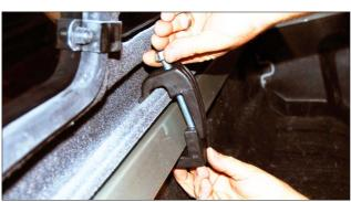
Loosely fit the three clamps to the flange as shown, to both sides.
