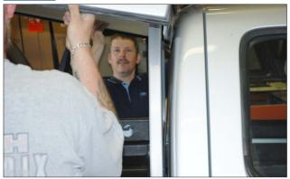
1 Lift the top onto the bed (over the ladder-rack if fitted). This is best achieved with one person at the rear door end and two people guiding the front of the top. Keep the rear end slightly raised until the hardtop is in position.
