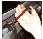
Push the rear light wires through the small hole under the loadbed rail.
