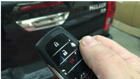
3. Close all of the doors and check that the canopy locks and unlocks with the vehicle's remote.
