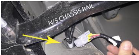
4. Take the wiring harness from the fitting kit then, from underneath the N/S rear of the vehicle, pass the grey plug up through this hole, into the light recess.
