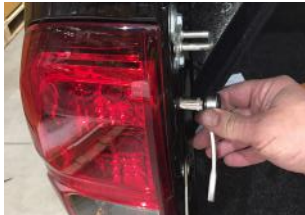
1. Remove the screws from the N/S/R light cluster.
