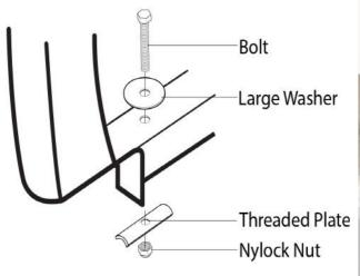
**16.** Insert the fixings as shown in the diagram, omitting the Nylock nut. Tighten to 6Nm.
