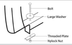
**17.** Bolt the hardtop (without nylock nut) to the vehicle as shown in the diagram and tighten to 6-8Nm.
