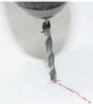
**16.** Complete the holes with a 9mm drill bit.
