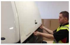
**13.** Align the top centrally and ensure that the seal under the hardtop door is just touching the tailgate.
