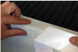
**21.** Carefully apply it to the tailgate where the door touches, rubbing outwards to remove any bubbles as you go.
