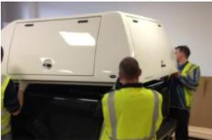
**10.** Lift the hardtop on to the vehicle.
