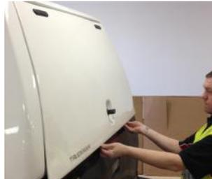
**11.** With the top now on the vehicle check that the seal under the rear door is just touching the tailgate.
