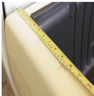
5. Measure from the front of the side rails, apply tape and make marks in the positions shown below.
