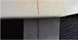
*Tip: Use masking tape & pencil. Continue the lines to the inside of the bed or liner to aid alignment later.*
