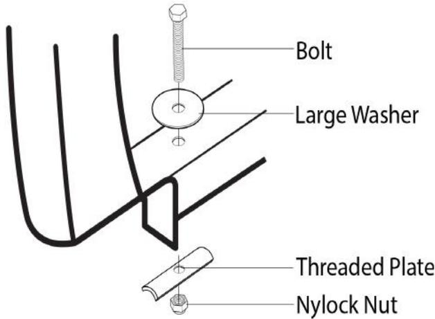
**16.** Insert the fixings as shown in the diagram, omitting the Nylock nut. Tighten to 6Nm.
