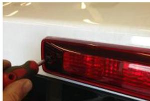
3. Unscrew the vehicle's third brake light and pull it away from the bodywork.
