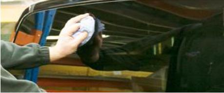
**8.** Thoroughly clean the vehicle's rear window and the hardtop's bulkhead window (if fitted).
