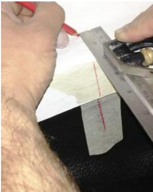
**13.** With the door closed, measure and mark the same dimensions as before onto the top (using Step 8's lines as a guide).
