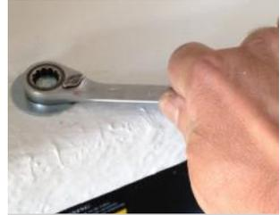
**17.** Now add the nylock nuts under the threaded plates and tighten, again to 6Nm.
