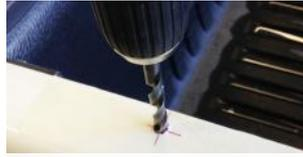
**6.** Drill a 3mm pilot hole 15mm from the inside edge of the rail. Drill again with a 9mm bit.
