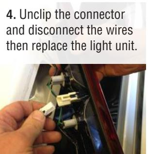
4. Unclip the connector and disconnect the wires then replace the light unit.
