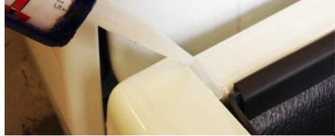
**9.** Fill the front corners of the bed with silicone sealant. (Where the side rails meet the front rail).
