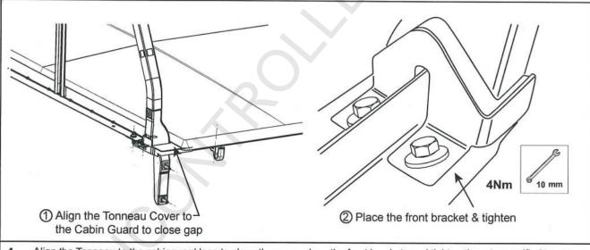
4. Align the Tonneau to the cabinguard legs to close the gaps, place the front brackets and tighten them to specified torque.
