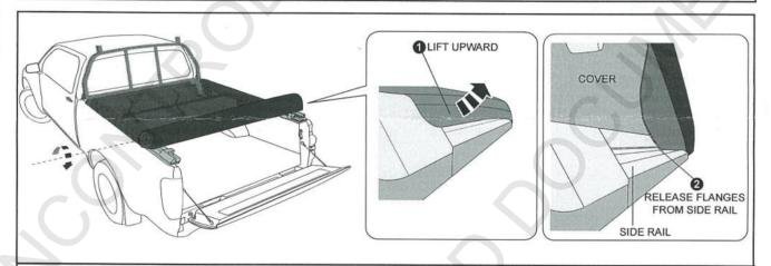
2. Working from the rear of the cover, grip and lift in an upward direction to release the flexible flanges fron the side rails
