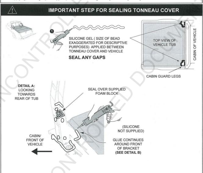
**14.** Seal all the gaps in and around cabin guard by applying Silicon gel (Not supplied). Allow the silicon gel to dry before any activity. This step is important, as it minimises leakage into the tray body in wet conditions.
