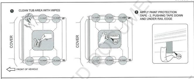
5. Clean the tub areas with alcohol wipes in the location marked 'CLAMP' on the side rail and apply the Paint Protection Tape – 2 (12 off).
