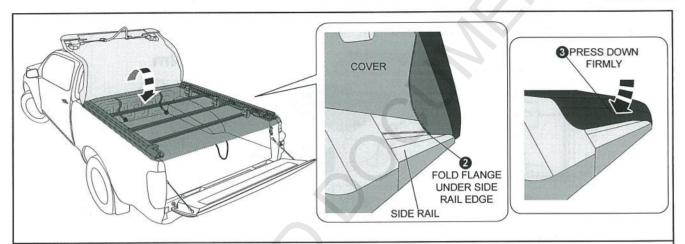
10. Roll cover over tub towards the rear of the vehicle. Fix the cover to the side rails by folding the flexible flanges on the cover outward and rolling them in under the edge of the side rails. To lock them in press firmly on the outside of the cover.
