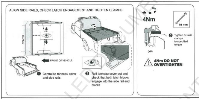
8. Centralise and align side rails. Check position of side rails by rolling Tonneau Cover out and ensuring that the side latches engage into side rail blocks on rear of Tonneau Cover. When correctly aligned lay cover back on the vehicle roof and tighten both front and rear side clamps to the torque specified.
