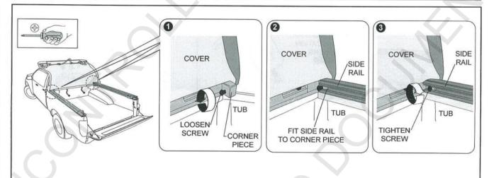
3. Loosen screws (ensuring they do not disengage from the backing nuts) on each side of the front rail corners. Engage the side rails into the front rail corner pieces ensuring they are fully seated. Tighten screws on both sides to firmly clamp the side rails to the front rail.
