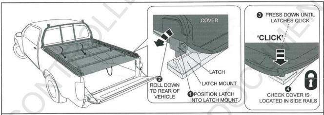
11. Position latches into stretch mounts. Holding the cover rail at the rear, roll towards the rear of the vehicle and down until latches click and are both locked into position. Ensure the flexible side flanges are fully seated into the side rails.
