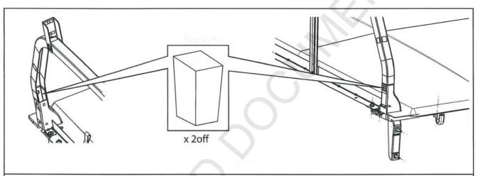
13. Plug the cabinguard holes using the cabinguard seal plug provided. Seal all the gaps in and around cabinguard by applying Silicon gel (Not supplied). Allow the silicon gel to dry before any activity.
