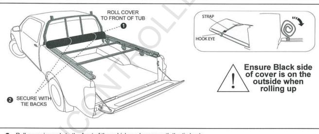
3. Roll cover inwards to the front of the vehicle and secure with the tie backs IMPORTANT: Ensure black side of the cover is on the outside when rolling up as it is UV protected
