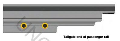
Remove the clamp and with a 6mm Allen wrench, turn both of the white nylon adjustment screws evenly. One complete turn of the adjustment screw= 1.5 mm of adjustment.
