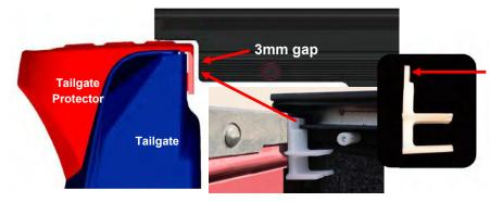
Move the rails to achieve the 3mm gap using the 3mm part at the top of the shipping bracket/spacing gauge. Make certain the rails do not move after measuring.
