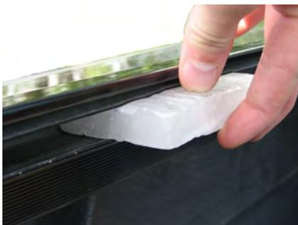
**IMPORTANT: NEVER spray any lubricant or cleaner in the rails. THIS WILL VOID YOUR WARRANTY.** The ball bearings are sealed and will not need any sort of lubricant or spray. If the rails do feel a little sticky, you may rub some Paraffin (candle) wax or bees wax along the rail until the wear in.
