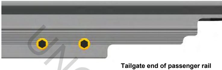
Remove the clamp and with a 6mm Allen wrench, turn both of the white nylon adjustment screws evenly. One complete turn of the adjustment screw = 1.5 mm of adjustment.
