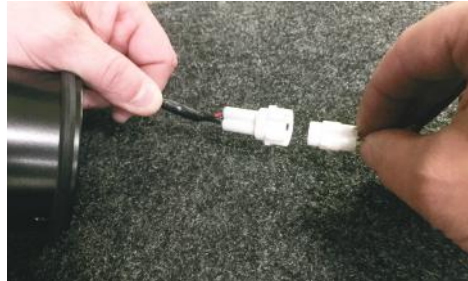
3. Connect the end of the intermediate harness (D) to the plug on the centre bar.
