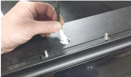
16. Feed the brake light plug through the 20mm hole in the Retrax rail
