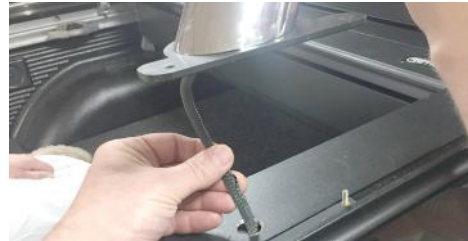
17. Lower the bar down onto the accessory studs, adjusting the plates if necessary.
