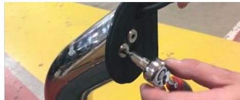
19. Remove the bar, apply thread lock to the screws then tighten, carefully maintaining the position of the plates.
