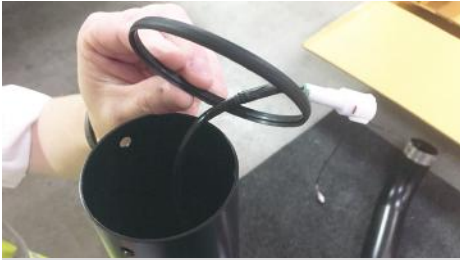
2. Fit a Joint cover O-ring (G) over each end of the centre section of the styling bar c/w brake light (A).
