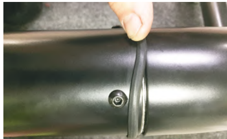
5. Fit the screws (using thread locking solution) then slide the joint cover O ring into place.
