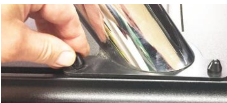
18. Remove the masking tape then fit the security nuts (L) with thread lock.
