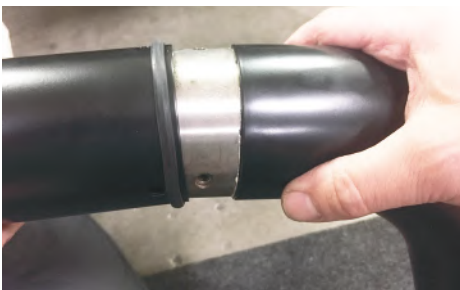
4. Fit the centre and R/H section of the bar together (ensuring brake light is facing towards the rear).
