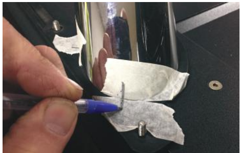
15. Use masking tape and a pen to mark the positions of the plates relative to the bar.
