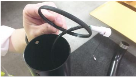
2. Fit a Joint cover O-ring (H) over each end of the centre section of the styling bar c/w brake light (A).
