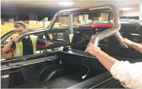
12. Lift the bar on to the Retrax.
