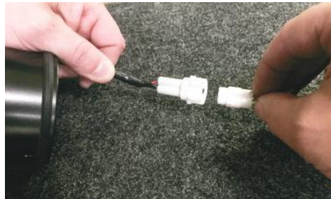
3. Connect the end of the intermediate harness to the plug on the centre bar.
