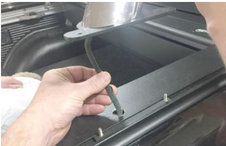
14. Lower the bar down onto the accessory studs, adjusting the plates if necessary.
