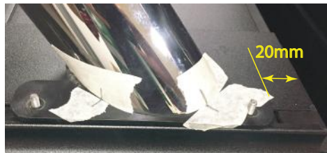
17. Refit the bar ensuring the front edge of the plates are 40mm from the front of the tonneau.
