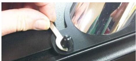
19. Use the spanner supplied to tighten the nuts.
