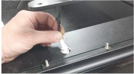
13. Feed the brake light plug through the 20mm hole in the Retrax rail
