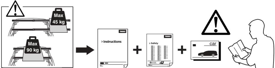
**GB** maximum load on Thule SlideBar = 90kg, or less if stated differently in roof rack- or car instruction manual.
