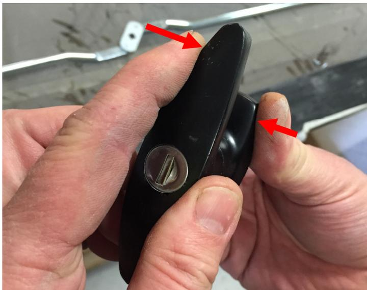
Rotate the handle fully clockwise against the foot before inserting into the mechanism and the door.
